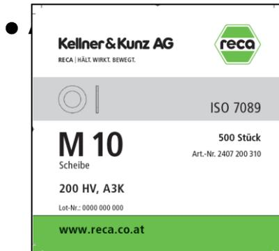
In order to identify the article clearly, the article label on the article packaging must include the **name and specification** for this article as shown on **supplier delivery note** as a minimum requirement.
