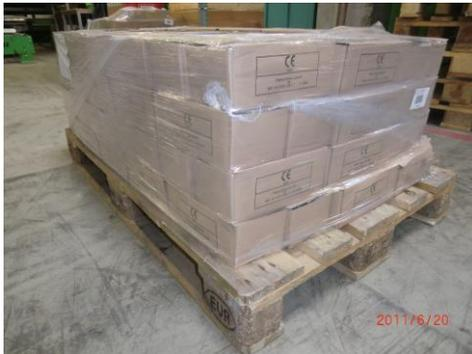
Articles with low weight, which are difficult to stack or slip easily on the pallet, need to be secured with **wrapping foil** as minimum protection against slipping.
