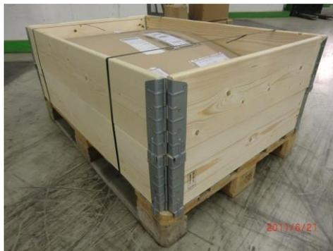
**Bulk packed goods** need to be secured with strapped **one-way pallet frames**.
